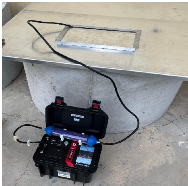
Figure 1. Experimental setup for radon permeability test using a portable radon analyzer on coated and uncoated concrete culvert samples.
