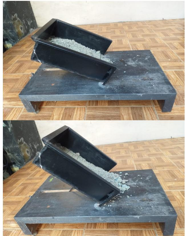
Figure 4. Measuring friction coefficient measuring instrument
