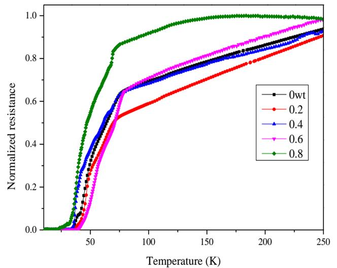
Figure 2. Normalized Resistance versus Temperature of Bi-2212 with CNT addition
