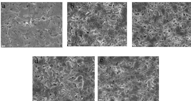
**Figure 3.** SEM surface morphology of CNT addition to Bi-2212 (a) 0.0, (b) 0.2, (c) 0.4, (d) 0.6, and (e) 0.8 wt. %
