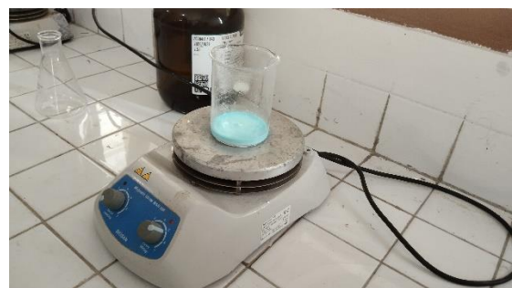
Figure 2. Process for Making Sol-Gel Solution
