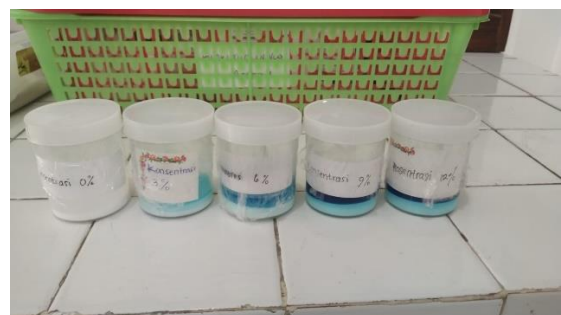
Figure 3. TiO 2 Solution with Concentrations of (0, 3, 6, 9, 12)%
