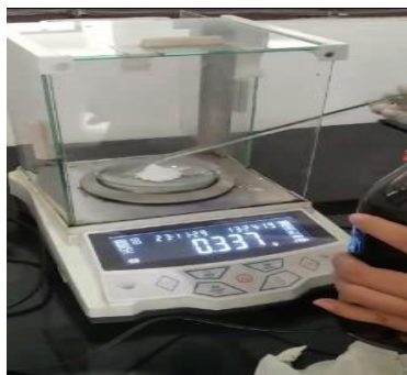
Figure 1. Process of Weighing Titanium and Cobalt
