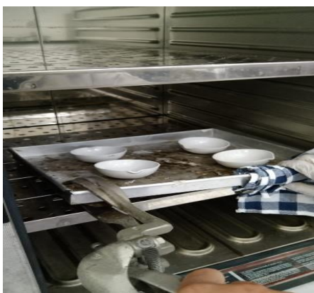
Figure 5. Heating the Glass Substrate
