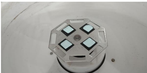
Figure 4. TiO 2 Thin Layer Deposition Process
