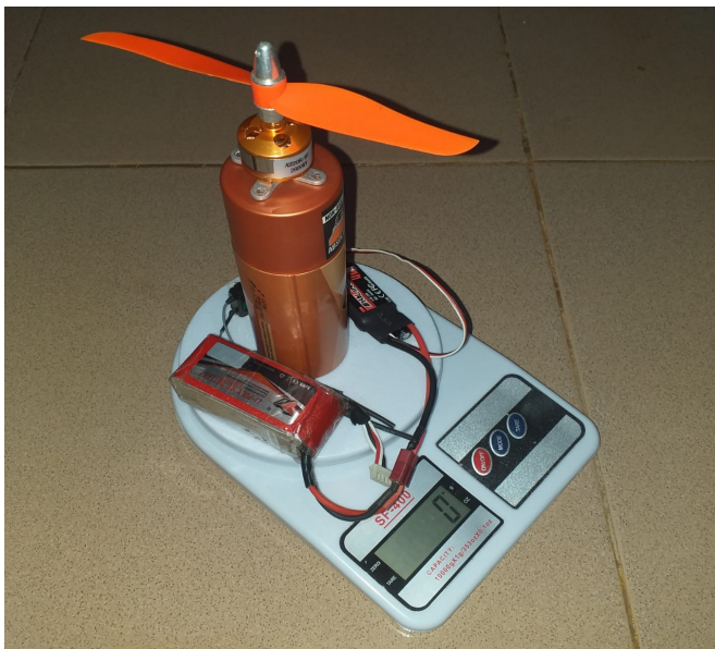
Figure 5. Measurement of the thrust force of a brushless motor with the SF-400 digital scale.
